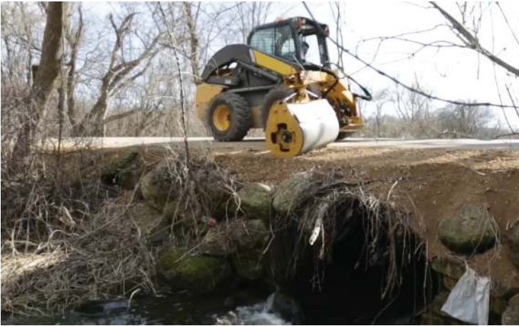
Offset feature allows operator to stay on the road while rolling and compacting shoulders and ditches.
